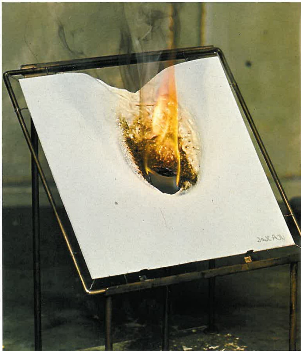
The Gas Flame Test described on page 22.
